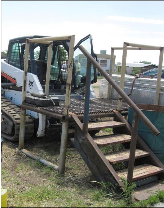
Figure 2. Steps and platform to access skidsteer.
