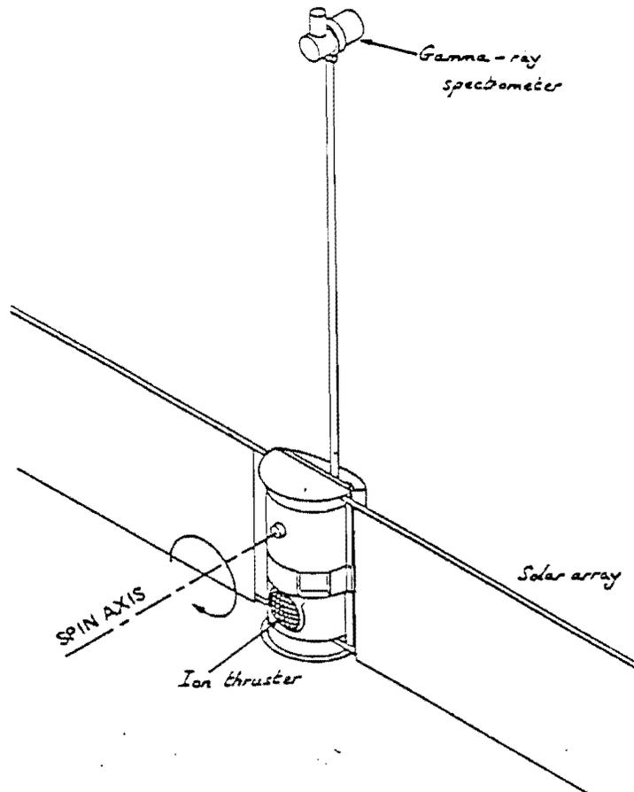
JPL's Proposed LGAS Spacecraft would be launched as a compact cylinder and would then unfurl large solar arrays to power its two ion thrusters
