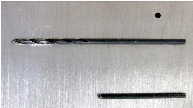
The drill bit rod was inserted into each hole and the thickness of the plate and bit was measured using a long micrometer (this thickness includes the protective tape).
