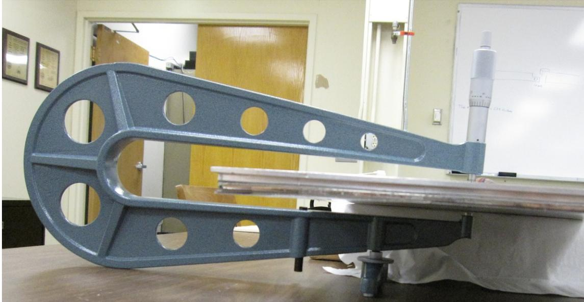
The measurement described above was repeated to establish random uncertainty in the measurement. It was found that the measurements repeated to within 0.002". So, the uncertainty of X is the root sum of the bias and random uncertainty, or
